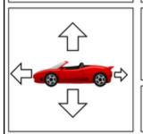
Forces Weight: 15 000 N Reaction Force: 15 000 N Driving Force: 15 000 N Air Resistance & Friction: 9000 N
