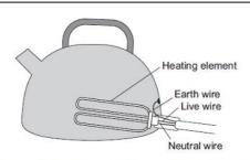
If a fault makes the metal case live, the earth wire and the fuse inside the plug protect anyone using the kettle from an electric shock.
