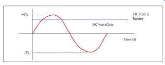
Alternating current changes direction and is mains electricity. Direct Current does not and is from a battery.
